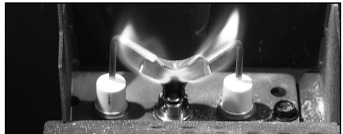
Figure 3.1 IPI Pilot Flame Patterns
